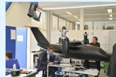
Figure 1 – The complex, densely instrumented tilt-rotor model manufactured by NLR (left); its installation in the ONERA S1MA wind tunnel (right). NICETRIP project.
