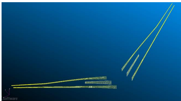
Fig. 2 Depiction of the wing structure in the FEM model. The elasticity of the front and rear spar is tuned for 10 percent tip deflection in 1g flight.
