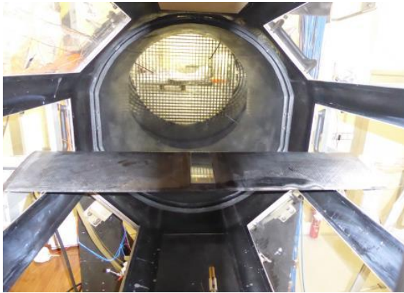
Fig. 1 NACA0012 airfoil model in ONERA S2L wind tunnel.
