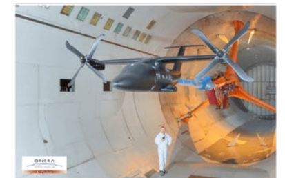
Figure 1 – The complex, densely instrumented tilt-rotor model manufactured by NLR (left); its installation in the ONERA S1MA wind tunnel (right). NICETRIP project.
