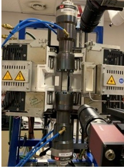
Fig. 5: High temperature set-up for testing composites
