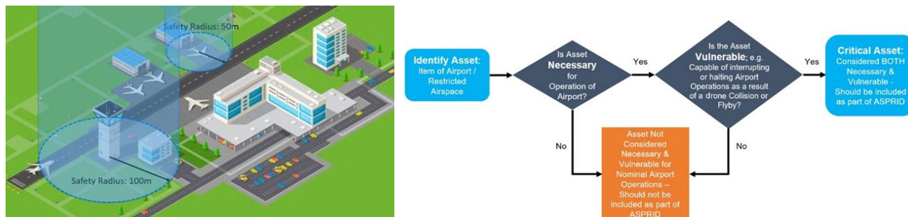
Figure 6 – Analysis of some specific threat scenarios (Fly-By or drone flying too close to an asset, Collision) and procedure for the assessment of critical assets
