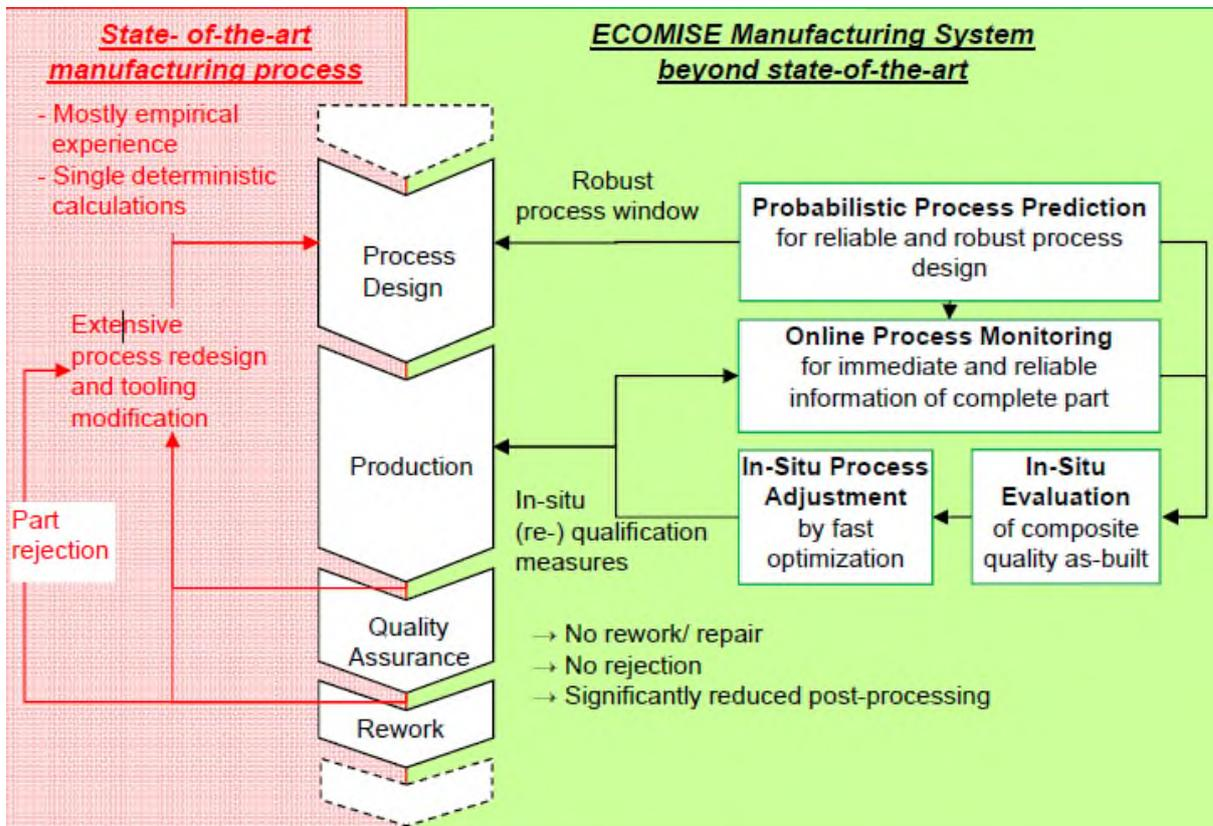
Figure 6 The ECOMISE manufacturing process
