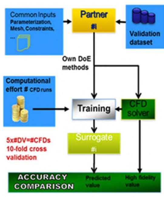
Figure 4 Surrogate models validation strategy (common inputs and dataset were used for surrogate validation). A 10-fold cross validation strategy has been applied, limiting the number of CFD runs to five times the number of design variables in the optimization problem
