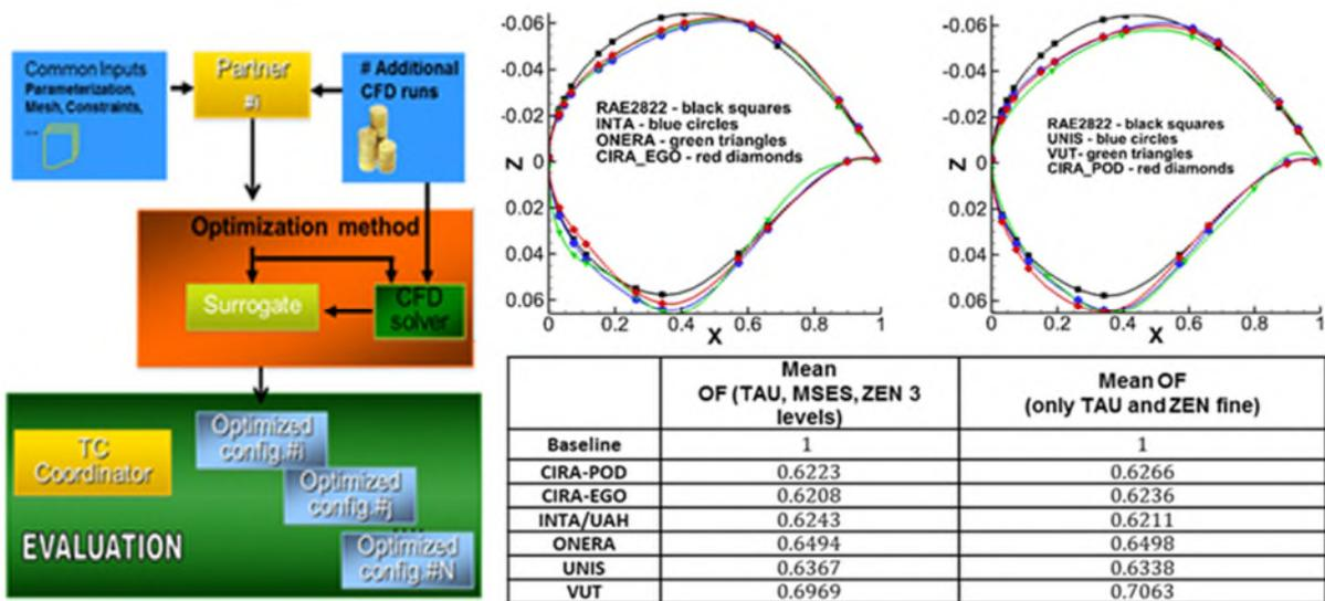
Figure 5 Flowchart of the SBGO comparison process (left) and optimization results for the RAE2822 test case(right). The flowchart shows how the comparison of the optimization results was performed and the table displays the mean objective function computed with different solvers (TAU, MSES and ZEN)
