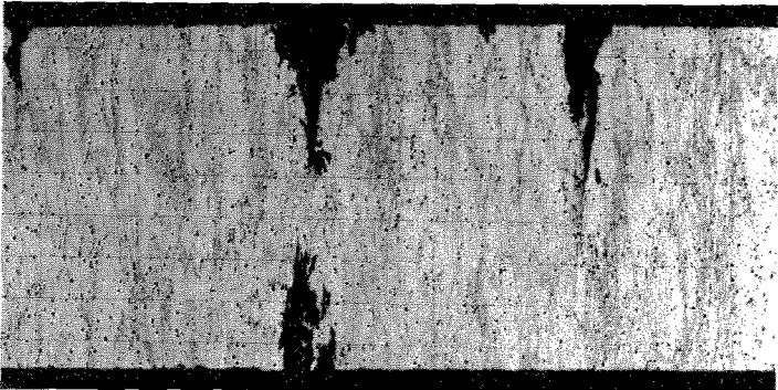
Fig 22 Sections of 7010 alloy test pieces given different quenching treatments, aged to a T73 condition and exposed to 3% NaCl by alternate immersion
