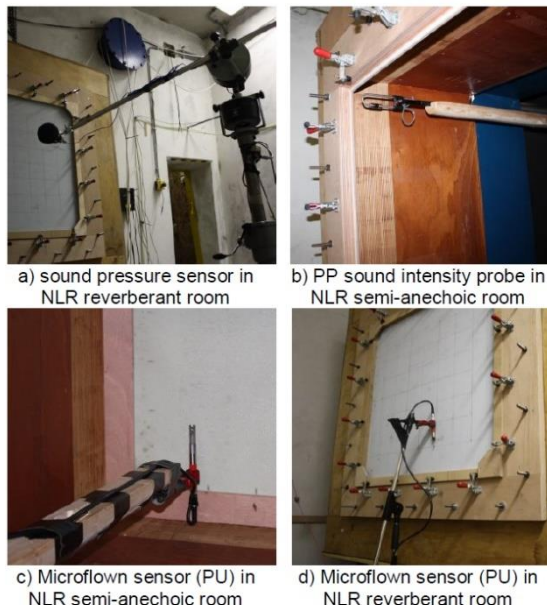
Figure 19: Sensors used for in-situ feasibility study
