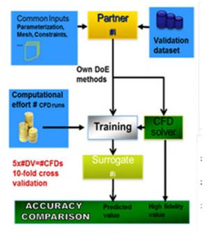
Figure 4 Surrogate models validation strategy (common inputs and dataset were used for surrogate validation). A 10-fold cross validation strategy has been applied, limiting the number of CFD runs to five times the number of design variables in the optimization problem
