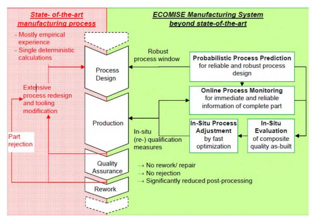
Figure 6 The ECOMISE manufacturing process
