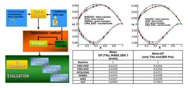
Figure 5 Flowchart of the SBGO comparison process (left) and optimization results for the RAE2822 test case(right). The flowchart shows how the comparison of the optimization results was performed and the table displays the mean objective function computed with different solvers (TAU, MSES and ZEN)
