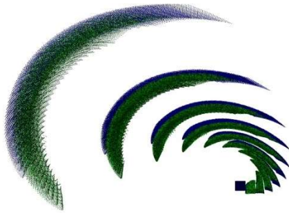
Chaff cloud evolution without turbulent dispersion behind a generic helicopter. Cylindrical chaff particles are initially aligned with the z-direction. FOI's results in green and NLR's in blue. The temporal increment between chaff clouds is 0.1 sec.
