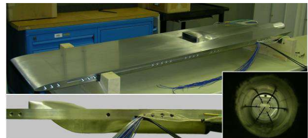
Fig. 2 Intake wind tunnel model with flat plate for parametric study in the DNW-KRG, Göttingen (top: 3D view, bottom left: side view, bottom right: view from the exit of the intake duct towards the measuring rake)
