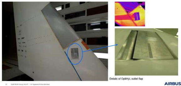
Fig. 4 Project OptiHyL in DNW-LLF wind tunnel: Hybrid Laminar Flow Control (HLFC) / Low Speed Wind Tunnel campaign of A320 VTP in DNW-LLF facility / The Netherlands
