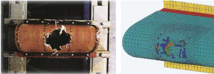
**Figure 8: Illustrations for the GoR Structures and Materials on computational modelling of bird strike and experimental validation, from SM/AG-24 on "Bird strikes"**
