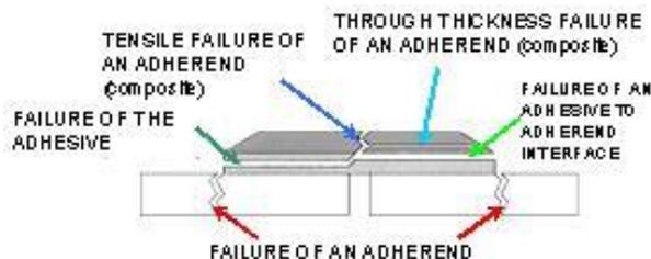
**Figure 9: Failure modes in adhesively bonded repair to be analysed within SM/AG32**
