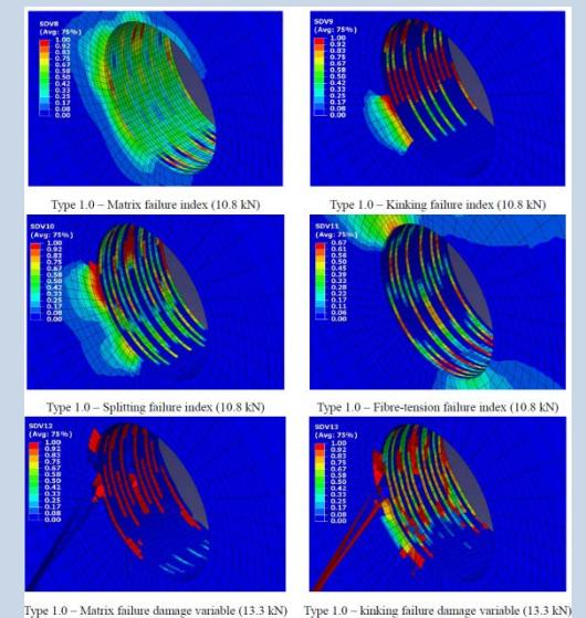
Numerical Analysis - progressive Damage in composite Joint
