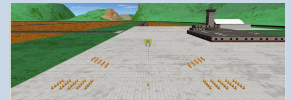
Precision Hover MTE: Example test course used in the piloted simulation trials
